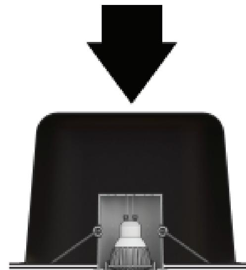
**3** Press down Loft Lid to secure in position
