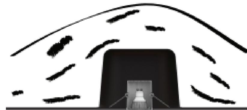
**4** Lay continuous insulation over Loft Lid
