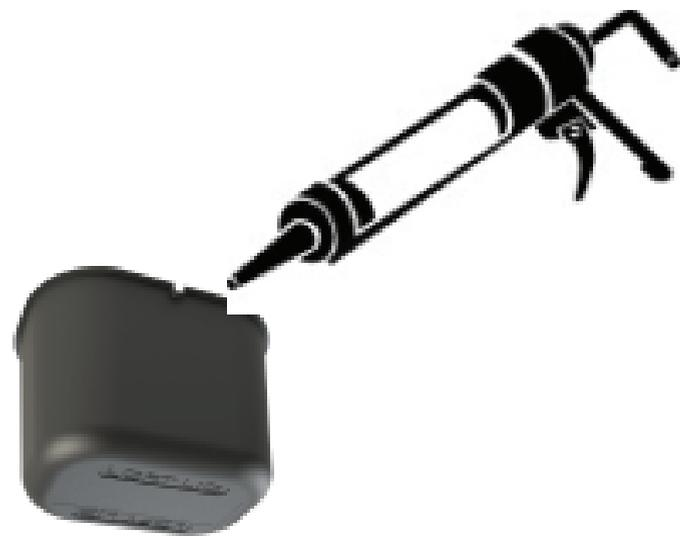
**2** Apply continuous layer of sealant/mastic to bottom lip
