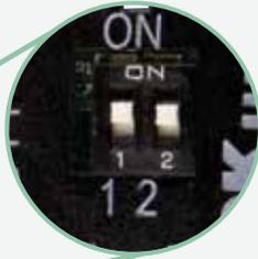
**1** Switch 1 allows the minimum brightness to be adjusted
